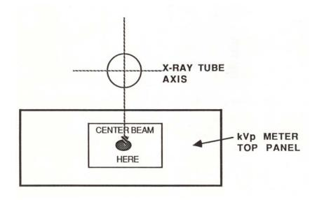
Figure 3-1. Detector Positioning
